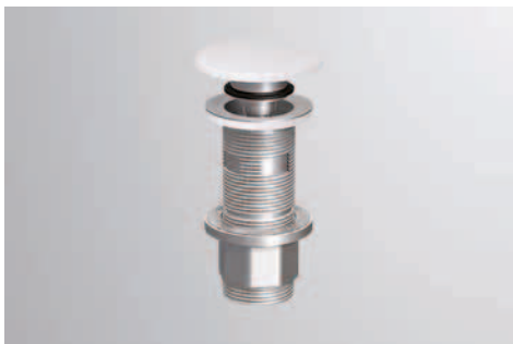
Drain valve, round, w/h/d 74/120/74 mm, Ø 1 1/4", with open/closed function, this basin requires an overflow, valve cap, white glazed
