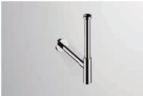
Bottle trap, w/h/d 45/419.5/390 mm, 1 1/4" connection thread, immersion tube, adjustable in height from 75 to 330 mm, adjustable depth from 90 to 390 mm
